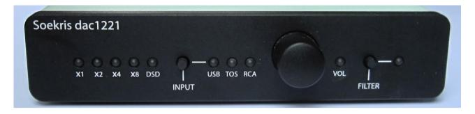
The LED's on the front indicates input sample rate, input source, reconstruction filters selected and a clip indicator.
