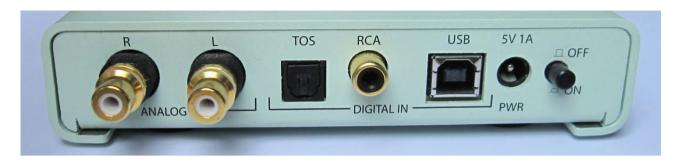
**Analog Out:** The dac1221 have single ended line out using RCA sockets, the red one marked "R" is for the right channel, the white one marked "L" is for the left channel.
